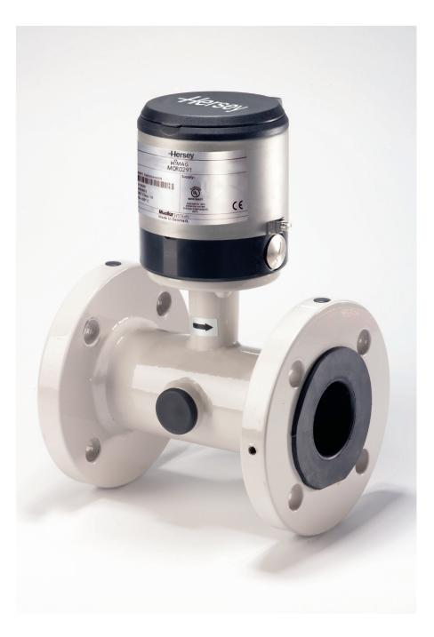
The HbMAG is is capable of exceptional accuracy even in non-standard piping configurations where the recommended minimum of 5 diameters upstream and 3 diameters downstream is not achievable due to the existing infrastructure.
