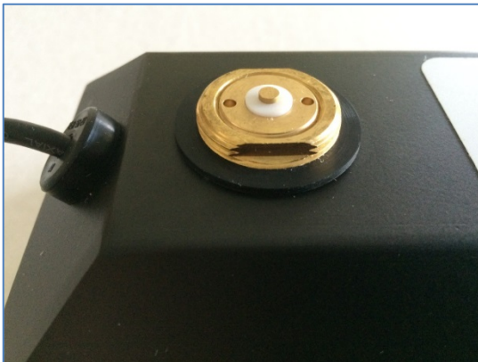
Properly seated gasket on base
