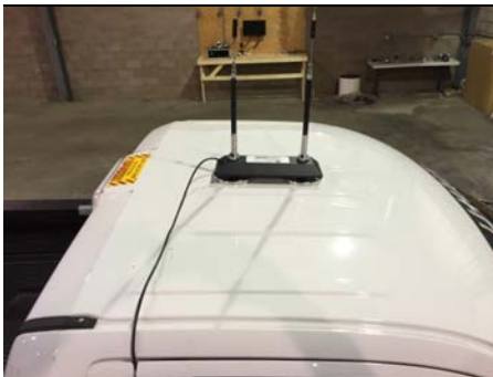
Figure 2 Cable routed through door
