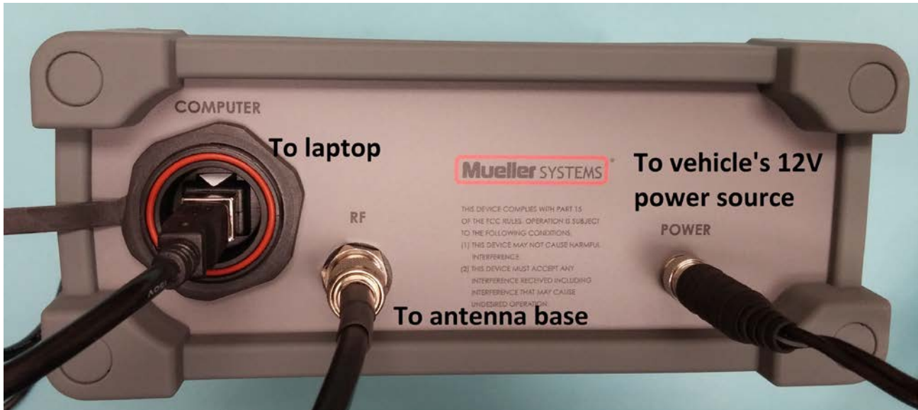
Figure 4 Rear of receiver showing connections
