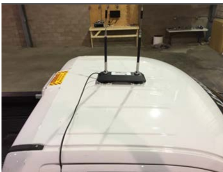
Figure 2 Cable routed through door
